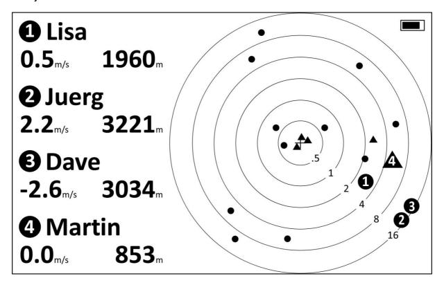
On the Buddy Screen you can see all paraglider and hang glider pilots who fly with a FLARM device and have been received by the XC Tracer Maxx in the last 5 minutes. Your position is in the middle of the circles, and from one circle to the next the distance (in kms) doubles.
