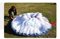
**Step 2.** Group LE reinforcements with the A tabs aligned, make sure the plastic reinforcements lay side by side.
